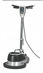
The FM Floor Maintainer has a rugged planetary drive system with helical-cut gears with an ultra smooth power trasmission. This versatile machine has an optional 4 gallon solution tank to help tackle larger jobs. The FM Floor Maintainer is built for decades of use with strengthened components such as the die cast aluminum housing, oversized bearings and seals in the gear box as well as large, durable wheels. The FM Floor Maintainer is available in 17 inch and 20 inch operating widths.
