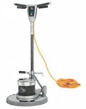
The 225FP is a corded floor care machine powered by a 1.5 HP UL approved high torque motor and equipped with a triple planetary gearbox. Available in two widths, 17" (43 cm) and 20" (51 cm), the 225FP can clean up to 6,000 square feet (557 square meters) and 7,000 square feet (650 square meters) of floors per hour, respectively. The machine comes standard with a pad holder and is also available with an optional 2.5 gallon (9,5 liter) solution tank.
