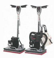
Totally enclosed 1 HP dual capacitor motor is fan cooled to eliminate overheating. 3450 orbits per minute sands faster than any other orbital sander available. Heavy duty cast aluminum main frame and pad driver plate for added strength. Bristle dust skirt and independent dust pickup fan for effective dust containment. Torque-less operation for enhanced operator comfort.
